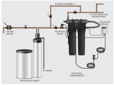
Figure 1. Typical Installation
