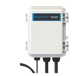
**SOLENOID CONNECTION MODULE:** Connects a NORMALLY CLOSED line voltage solenoid valve to the system. On a non-monitored system, the solenoid will only close on a lamp failure error. On a monitored system, the solenoid is closed when the UV level drops below 50%. Also note that in cases where emergency use of untreated water is required, the controller can be placed into a manual override mode allowing for the flow of water in an alarm condition. Order PN **40040006**.
