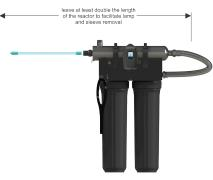
Figure 3. Lamp Removal Spacing
