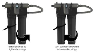
Figure 5. Cartridge Removal
