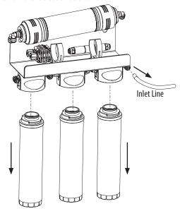
**2.** Disconnect all 3 cartridges and replace them with the blank sanitization cartridges included in this kit. Disconnect the inlet line from the system and drain excess water into a pail.
