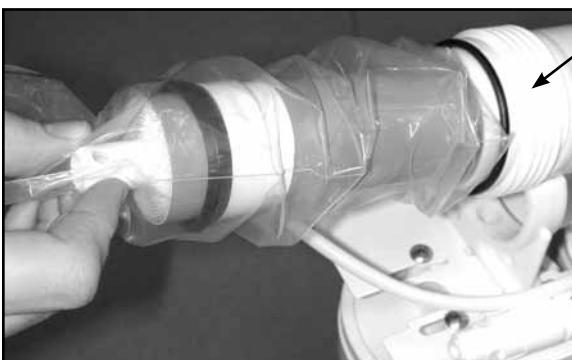
Figure 8B - Installing membrane - Remove cap
